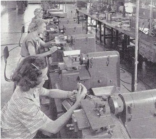
Our own automatic watch making machines designed and manufactured by Gruen for precision facing and recessing operations, at Norwood.
