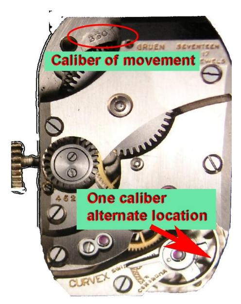
Figure 3 - Annotated Gruen Caliber 330 Movement
