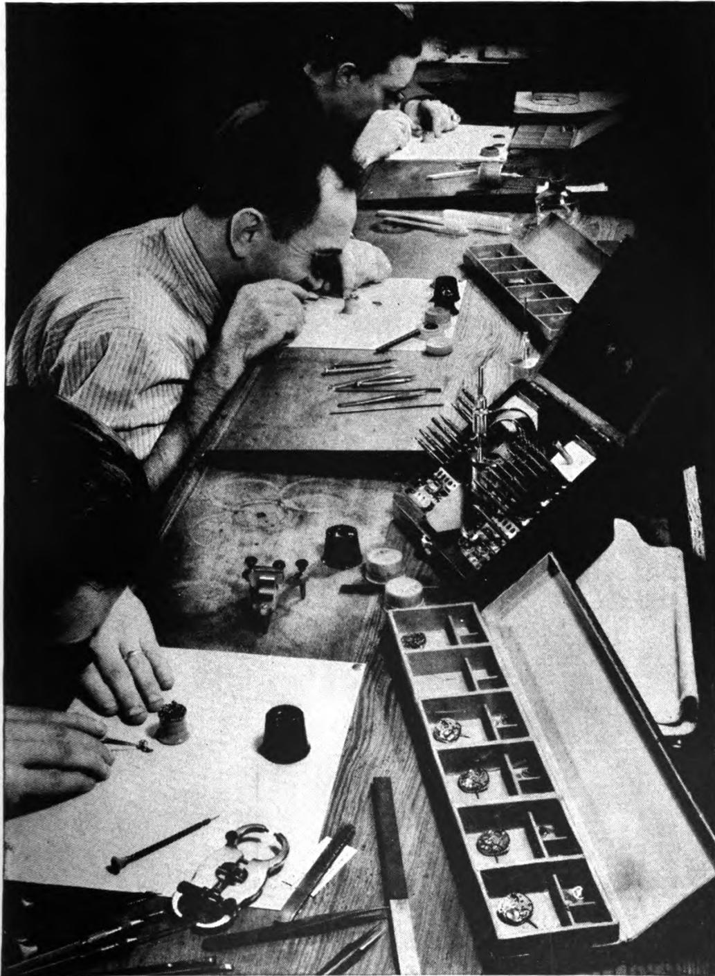
The assembly line. The ebauche moves to five watchmakers who assemble (1) the train; (2) the winding mechanism; (3) barrel and bridge; (4) escapement and (5) dial train and hands.
